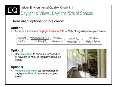
For <u>Option 1</u>, calculate a daylighting factor of 2% in 75% of regularly occupied spaces using the <u>glazing factor calculation</u>; include the area of each type of glazing (sidelighting and toplighting), the square feet of occupied area, and the visible light transmittance ( $T_{vis}$ ) for each glazing type.
