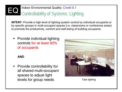
Design the building interior with a high level of lighting system control for the individual occupants, as well as lighting system controllability for multi-occupant spaces. Include integration of lighting systems controllability into the overall lighting design in order to provide both ambient and task lighting that will promote occupant comfort and productivity, while keeping energy use at a minimum.
