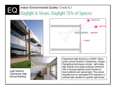
The diagram on the top right demonstrates how the light shelf is designed to block the summer sun from directly entering the building and instead, reflect it onto the ceiling of the interior in order to maximize the available light. In the winter, the sun's path is at a lower position in the Southern sky and is allowed to enter the building in order to provide light and an additional heat source for the cooler season.
