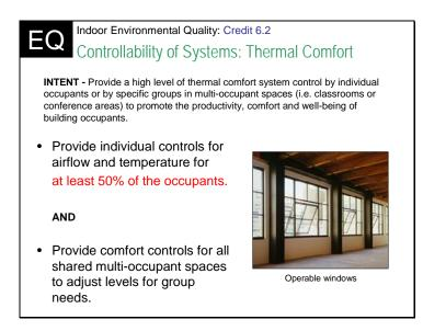
Credit 6.2 requires that thermal comfort be controllable by the occupants. Building design should included individual comfort controls, as well as comfort controls for groups in multi-occupant spaces. Individual adjustments may involve individual thermostat controls, local diffusers at floor, desk or overhead levels, or control of individual radiant panels. There may also be other means of control integrated into overall thermal comfort and energy systems in the building design.
