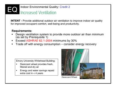
In order to achieve this credit for <u>mechanically vented spaces</u>, the outdoor ventilation rates to all occupied spaces must be increased by 30% above the minimum rates required by ASHRAE Standard 62.1-2004. One approach is to use heat recovery in order to minimize the additional energy consumption associated with higher ventilation rates.
