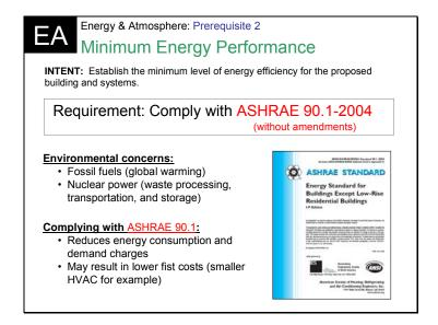
Maximize energy performance as much as possible through lighting, HVAC, an air tight and insulated building envelope, and water heating systems. The components of ASHRAE include building envelope, heating, ventilating, air conditioning, service water heating, power and lighting. ASHRAE 90.1 is the energy standard for many states, so attaining this credit usually requires no extra planning.
